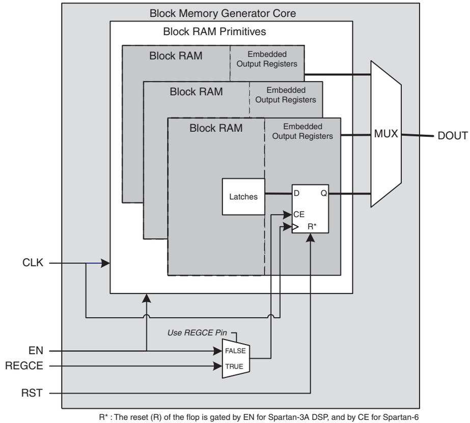
Figure 42: Virtex-5 FPGA Block Memory Generated with Register Port [A|B] Output of Memory Primitives Enabled
