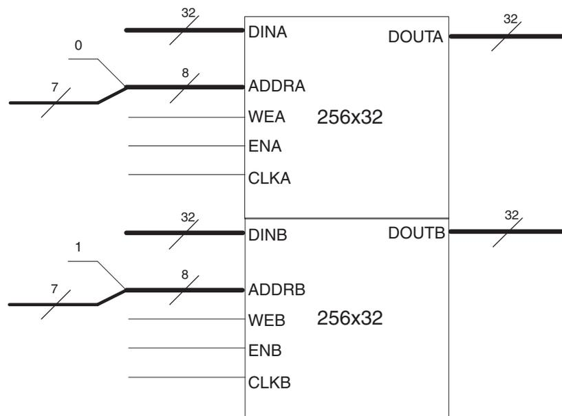
**Figure 37: Construction of Two Independent 128x32 Memories using a Single 256x32 Memory**
