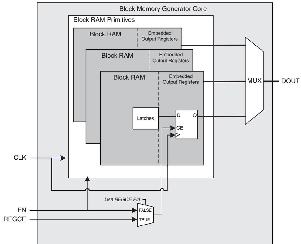
Figure 48: Spartan-6 or Spartan-3A DSP Block Memory Generated with Register Port [A|B] Output of Memory Primitives Enabled (No RST)
