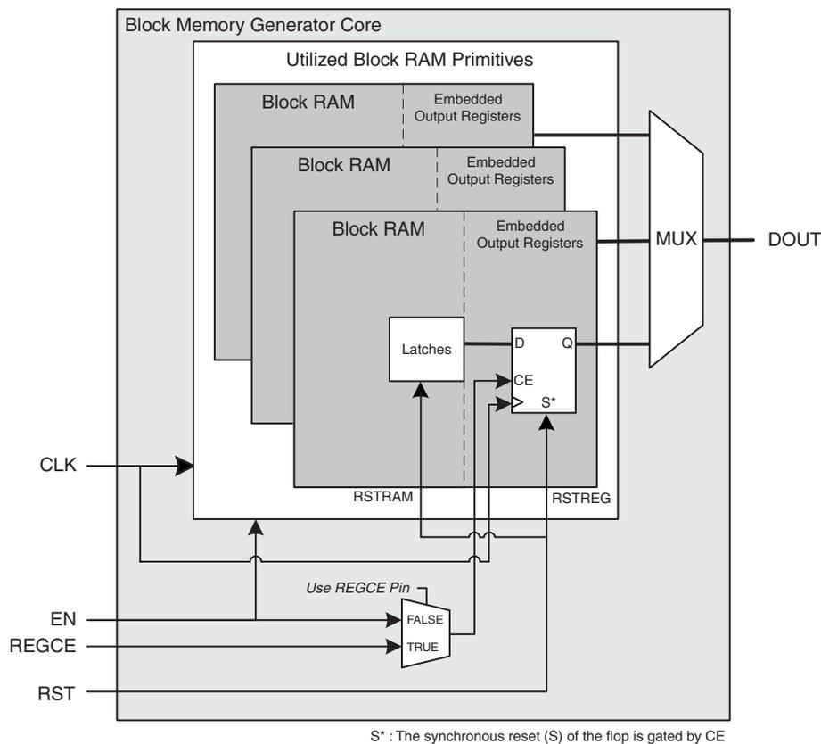
**Figure 41: Virtex-6 FPGA Block Memory Generated with Register Port [A|B] Output of Memory Primitives Enabled and with Special Reset Behavior**
