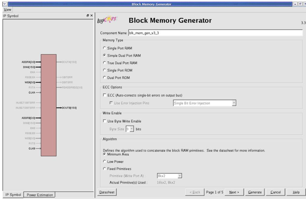
Figure 31: Block Memory Generator Main Screen
