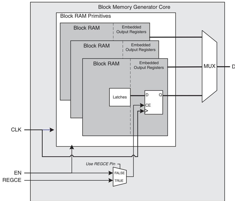
Figure 43: Virtex-4 Block Memory Generated with only Register Port [A | B] Output of Memory Primitives Enabled
