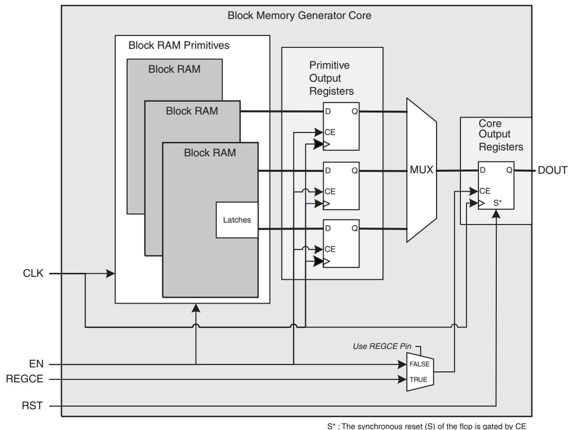
Figure 17: Spartan-3 Block Memory: Register Port [AIB] Outputs of Memory Primitives and Memory Core Options Enabled
