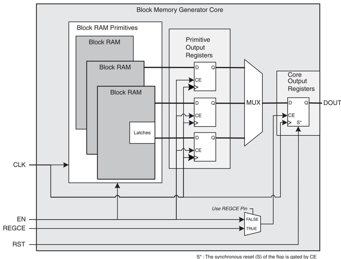
Figure 53: Spartan-3 Block Memory Generated with Register Port [A|B] Output of Memory Primitives and Register Port [A|B] Output of Memory Core Options Enabled
