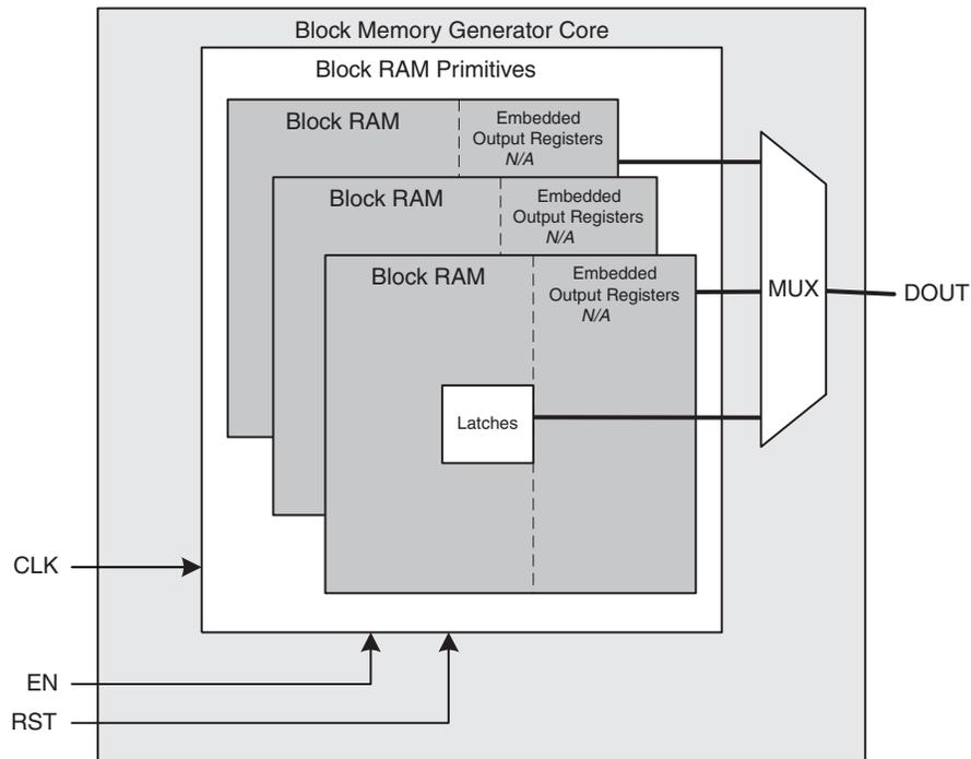
Figure 52: Spartan-6 or Spartan-3A DSP Block Memory Generated with No Output Port Registers Enabled
