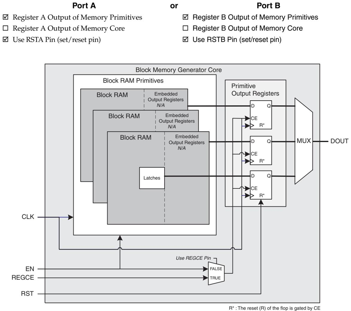
**Figure 44: Virtex-4 Block Memory Generated with Register Output of Memory Primitives and Use RST[A|B] Pin Options Enabled**
