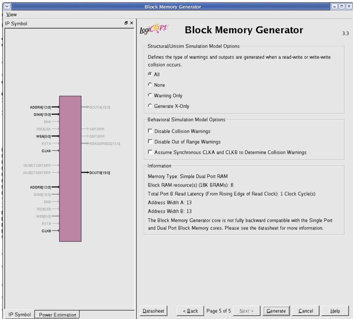
Figure 35: Simulation Model Options and Information Screen
