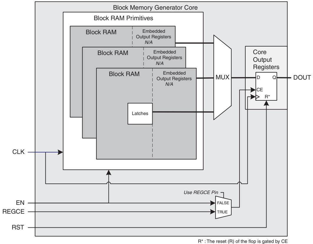
Figure 45: Virtex-6, Virtex-5, or Virtex-4 FPGA Block Memory Generated with Register Port [A|B] Output of Memory Core Enabled
