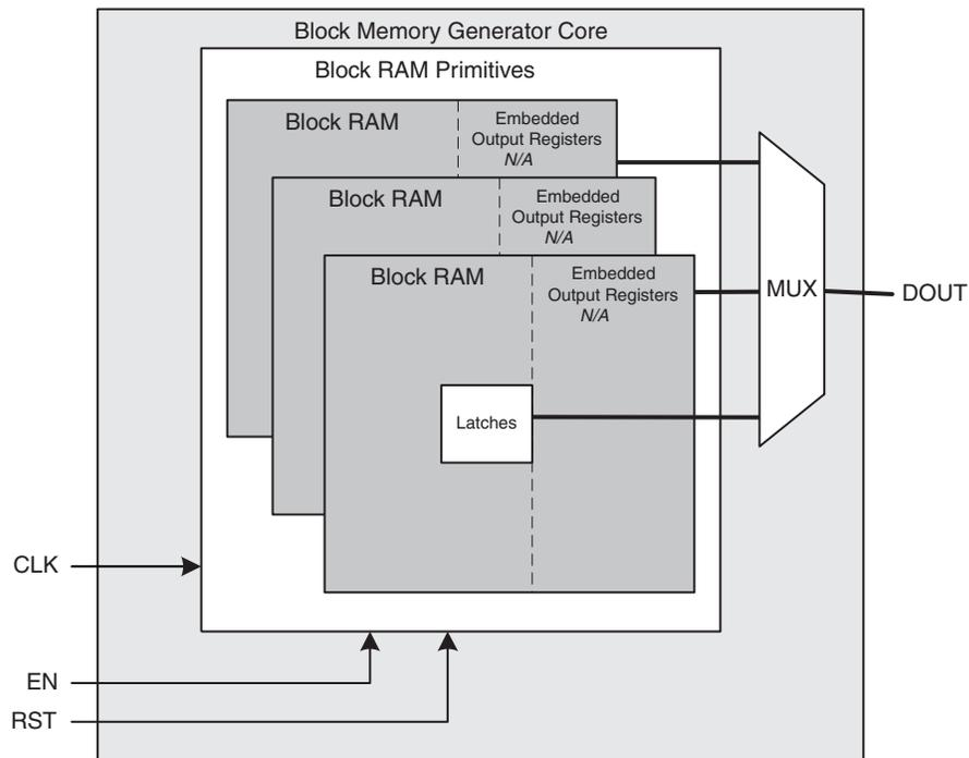
Figure 46: Virtex-6, Virtex-5 or Virtex-4 Block Memory Generated with No Output Registers Enabled
