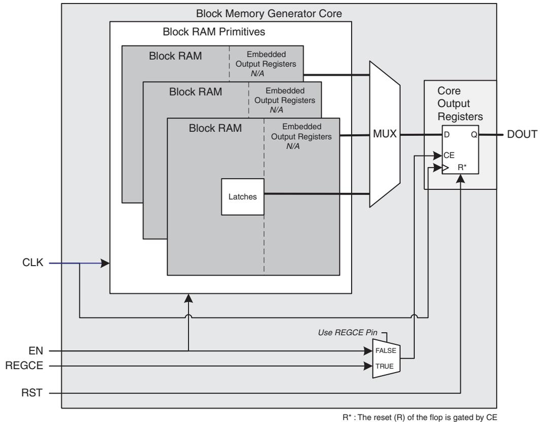
**Figure 51: Spartan-6 or Spartan-3A DSP Block Memory Generated with Register Port [A|B] Output of Memory Core Enabled**
