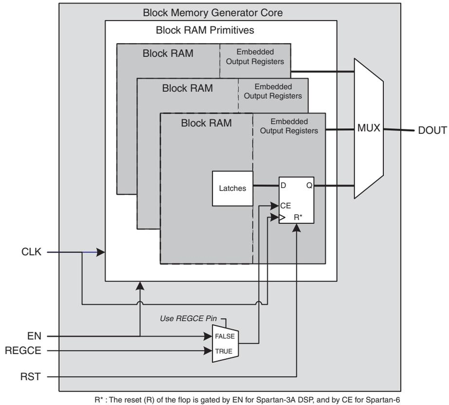
**Figure 50: Spartan-6 or Spartan-3A DSP Block Memory Generated with Register Port [AIB] Gated by EN in Spartan-3A DSP and by CE in Spartan-6 Output of Memory Primitives, Use RST[AIB] Pin Options (With RST), and Special Reset Behavior Enabled**
