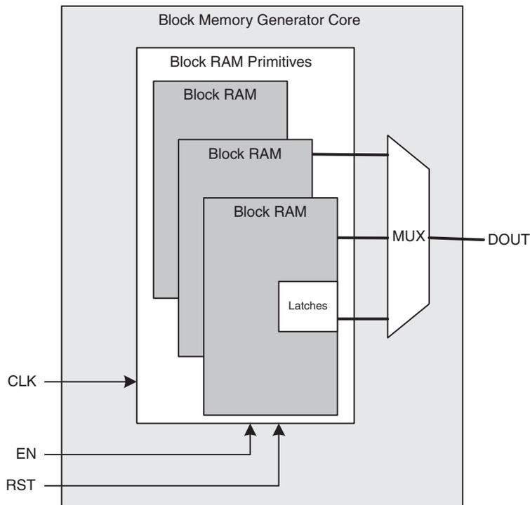
Figure 56: Spartan-3 Block Memory Generated with No Output Registers Enabled
