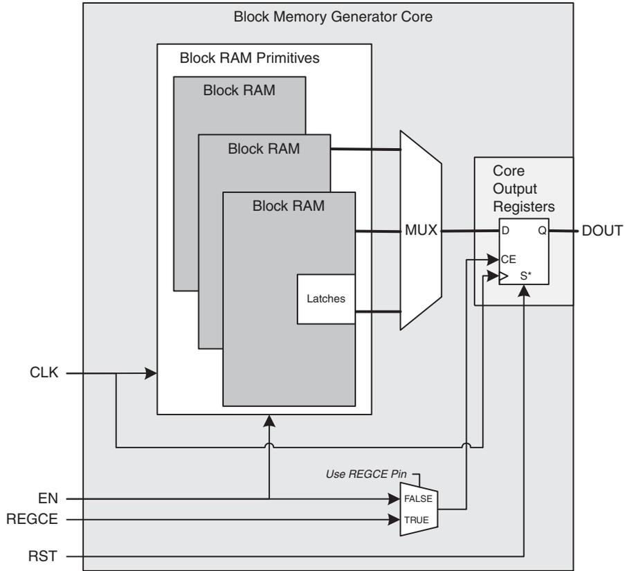
S\* : The synchronous reset (S) of the flop is gated by CE
