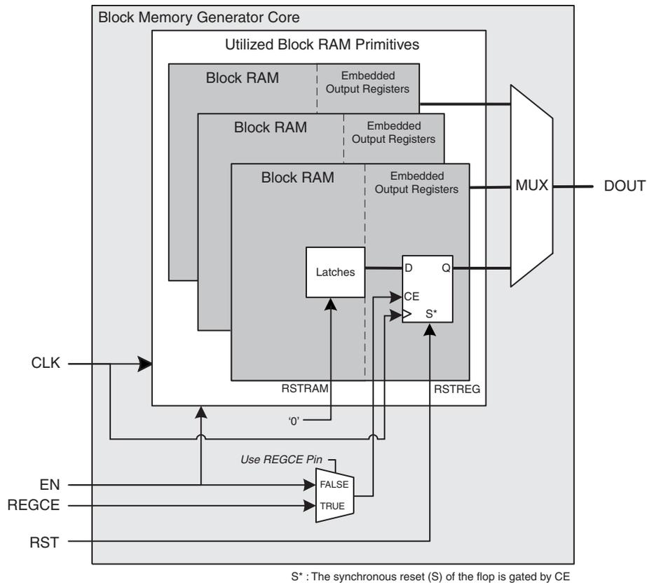
**Figure 40: Virtex-6 FPGA Block Memory Generated with Register Port [AIB] Output of Memory Primitives Enabled and without Special Reset Behavior**
