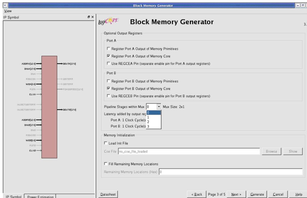
Figure 33: Output Registers and Memory Initialization Screen
