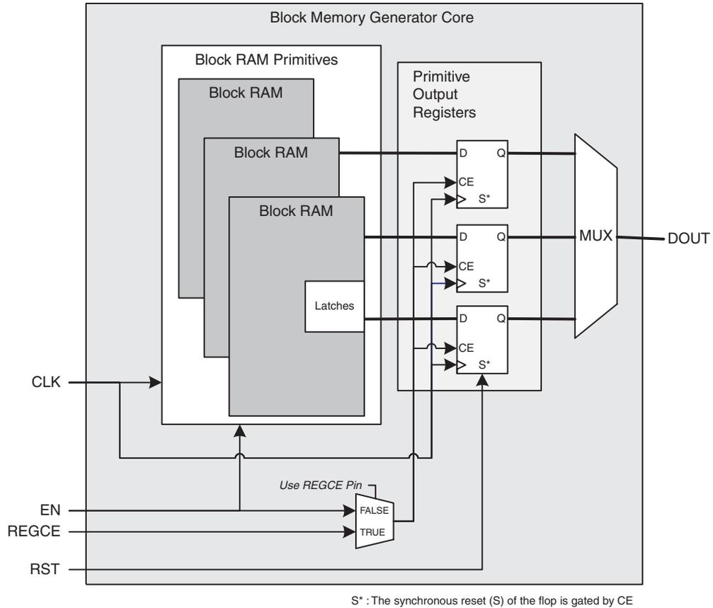
Figure 54: Spartan-3 Block Memory Generated with Register Port [A|B] Output of Memory Primitives Enabled
