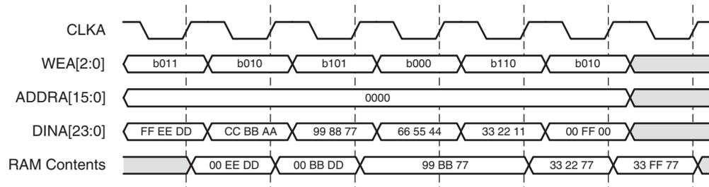
Figure 14: Byte-write Example
