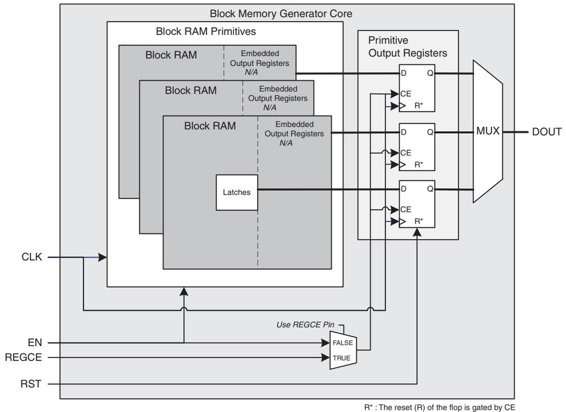
**Figure 49: Spartan-6 or Spartan-3A DSP Block Memory Generated with Register Port [AIB] Output of Memory Primitives, Use RST[AIB] Pin Options (With RST), without Special Reset Behavior**
