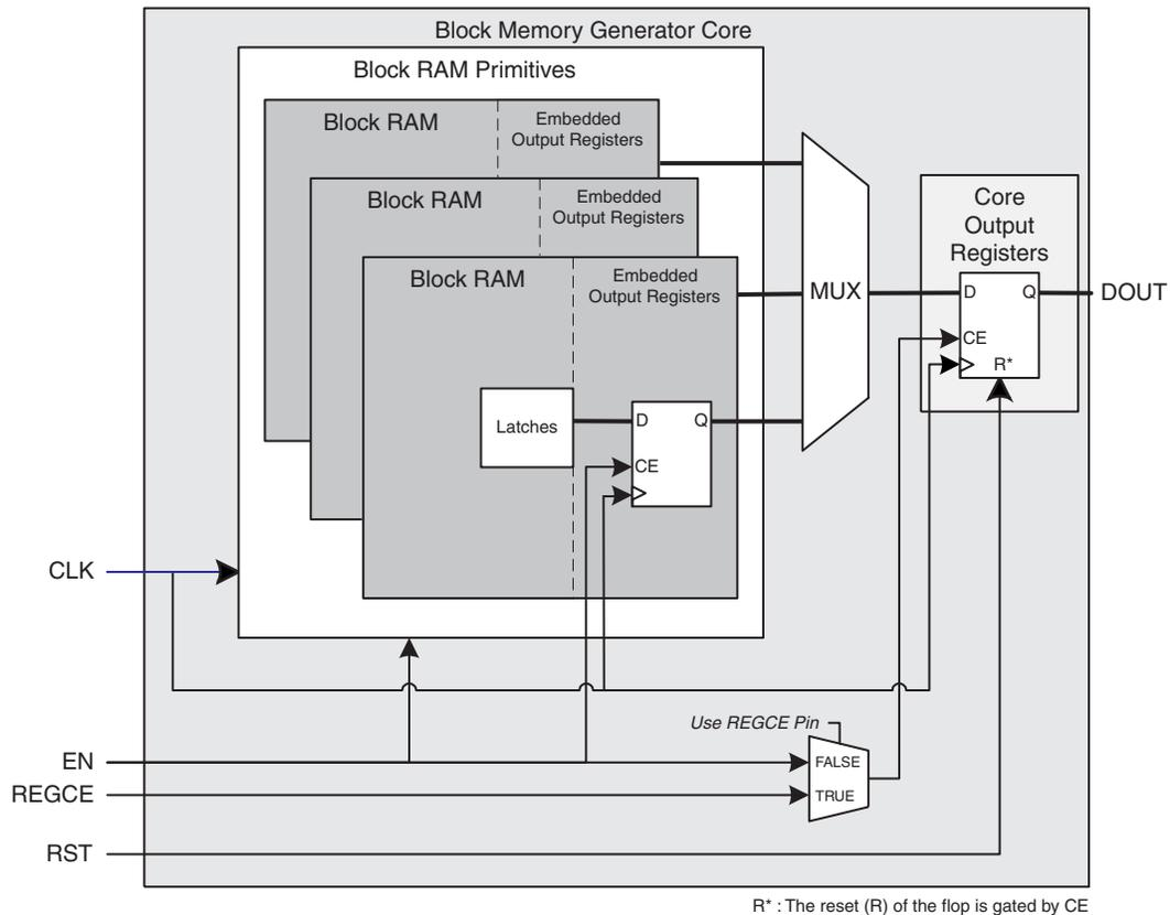
Figure 47: Spartan-6 or Spartan-3A DSP Block Memory Generated with Register Port [A|B] Output of Memory Primitives and Register Port [A|B] Output of Memory Core Enabled
