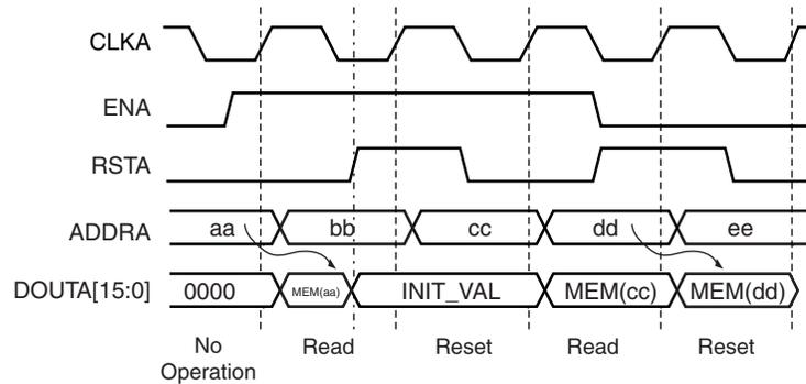
Figure 28: Asynchronous Reset
