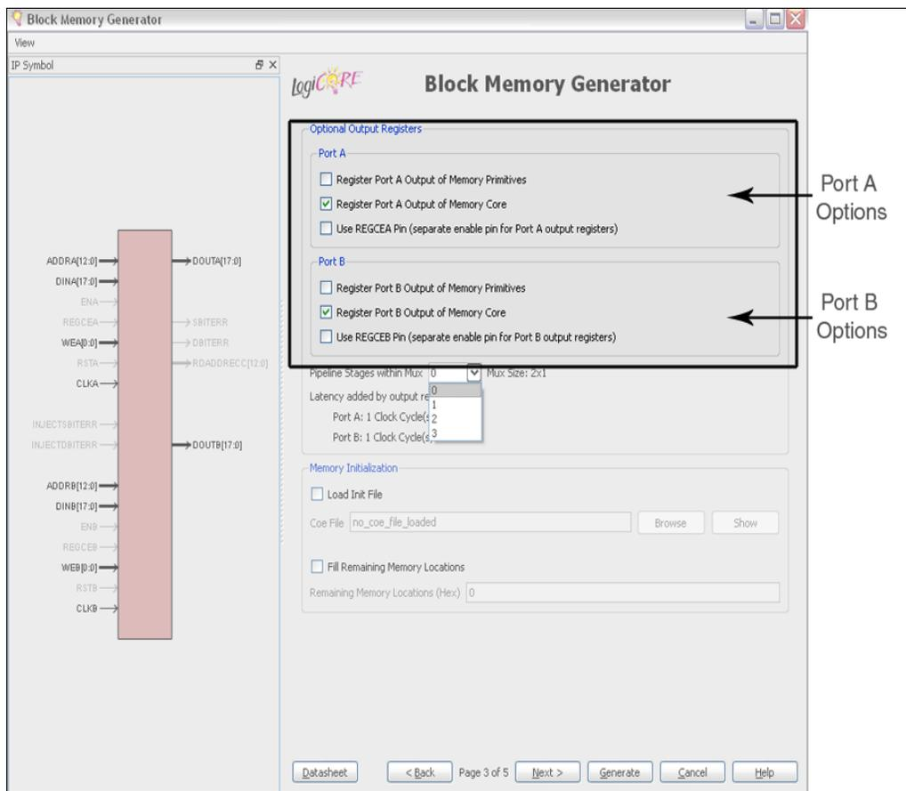
Figure 38: Optional Output Registers Section
