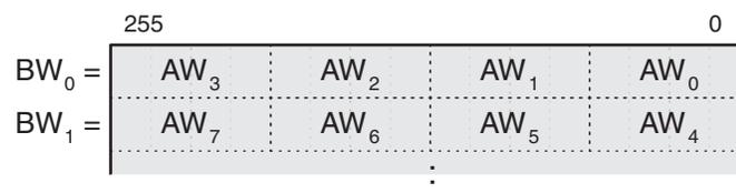
**Figure 13: Read-to-Write Aspect Ratio Example Memory Map**
